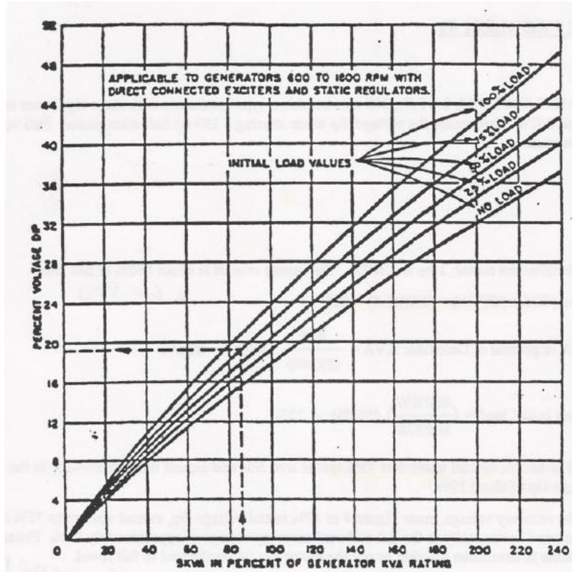
Voltage Dip with Motor Starting Loads
