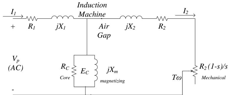
Some models combine the two components of  $R_2$  into one value of  $R_2/s$ . Mathematically that is correct, but in application the winding is separated from the mechanical component.
