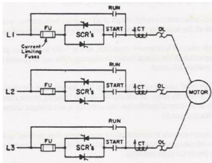
If the actual motor speed during acceleration lags the desired motor speed by more than 15% of the full load speed for a period of 5 seconds, this indicates that the load is too great for the available torque. Then the SCR's are turned off and the start contactor is de-energized.
