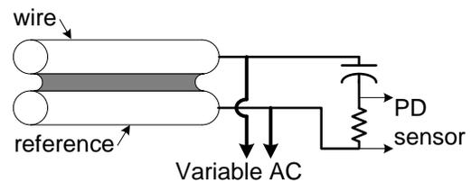
The signal is detected and processed for presentation, often on an oscilloscope type display. The partial discharge signal is given in millivolts or picocoulombs. A filter isolates the frequency of the discharges to the desired
