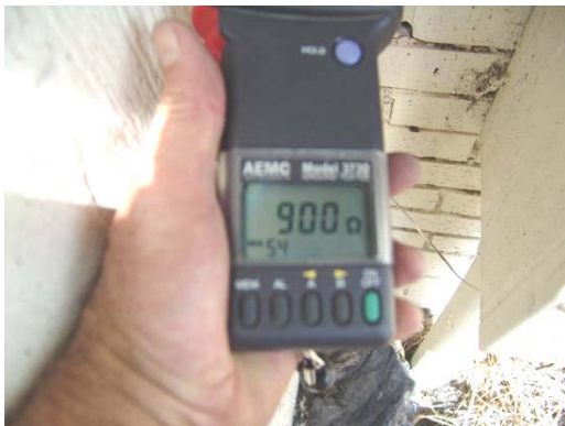
Figure 7: Ground resistance measurement
